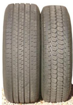
figure 3 Measurement tyres P1 (SRTT, left) and H1 (Avon Supervan AV4, right)
